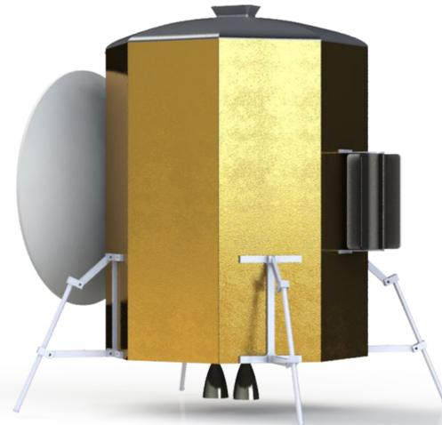
Figure 3: Up to date CAD model of the LITE spacecraft. Notable features visible from the exterior are the radioisotope thermoelectric generator (RTG), communications dish, thrusters, landing legs, sample catch funnel, and the environmental protection skin on the exterior of the primary structure.
