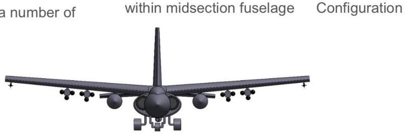
Aft Landing gear when stowed extends past the fuselage to act as additional cushion in the event of a belly landing
